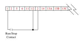
To add a potentiometer for speed control, change Parameter #5 (Standard Speed Source) to 0-10 VDC (03).
